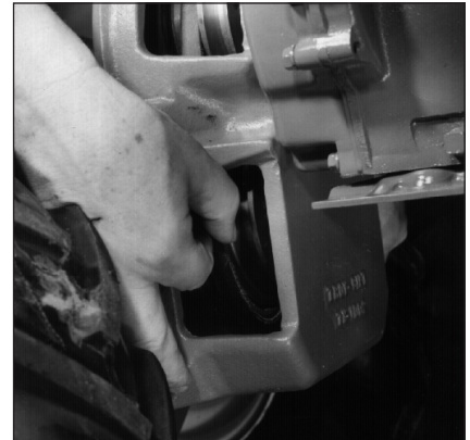
Figure 5-17: First move belt off the lower pulley.
